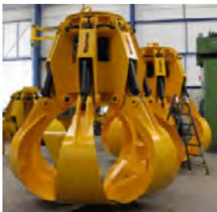
Should the product be heavy or compacted, of big granulation or sometimes mixed with light products or plastic packages, the grab works at a lower or higher speed, regulating the penetration force required and with the adequate dragging of the material. It changes the speed and regulates the pressure according to the material characteristics in each moment, the company says.
