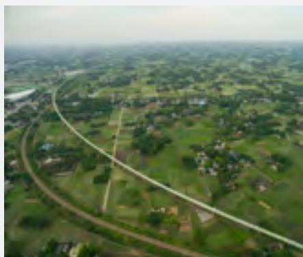
BEUMER Group produces curved belt conveyors as open troughed or pipe conveyors, which are capable of transporting large quantities of bulk material from the quarry to the works or port cost effectively. They overcome long distances, steep gradients and tight curves, and can be individually matched to the particular task and topography. The pipe conveyors avoid any contact of the product with the environment and vice versa.
