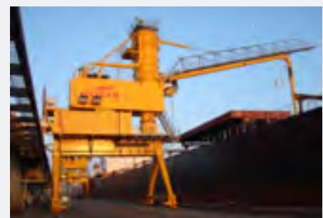
VIGAN NIV-TYPE SHIP UNLOADER OF 600 T/H INSTALLED IN TAIWAN IN 2018 AND IN THE BACKGROUND IS THE VIGAN NIV 600 T/H INSTALLED IN 2014
