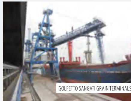
A mechanical shiploader, TRANSLOAD can be stationary or mobile on rails or wheels.
