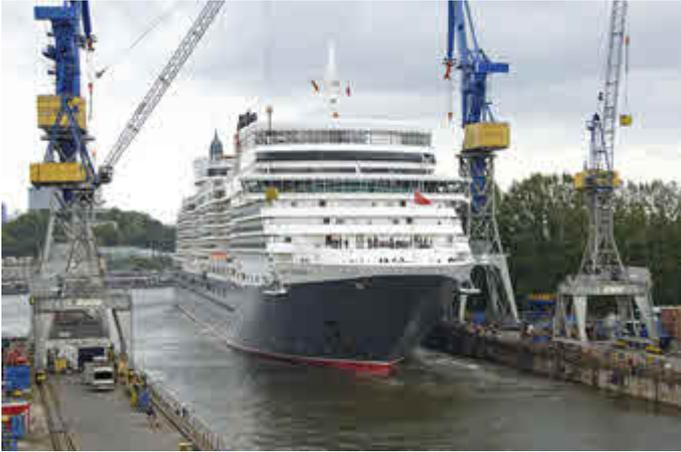
Cunard's flagship will undergo an extensive work scope that includes new cabins, modifications to the bridge wing, the installation of new bulkheads for improved damage stability as well as modifications to the vessel's tanks.
