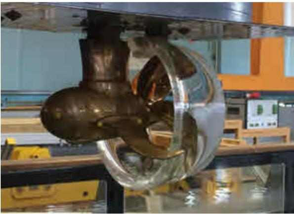
The Schottel VarioDuct SDV45 features optimally designed propeller geometries for "outstanding performance characteristics". Given the same propulsive power, Schottel claims it has a greater bollard pull than the thrust of previous nozzles and, at the same time, offers considerably greater efficiency in the medium and high speed range.
