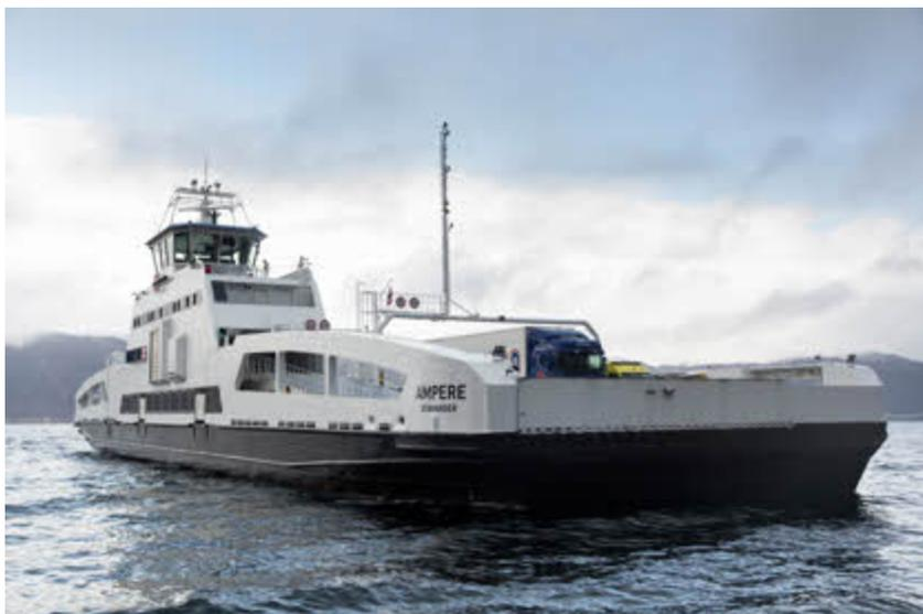
The ship's energy storage system is charged at each side of the crossing, with a shore connection to the local grid. Due to the harsh winter conditions in Finland, the ferry will have the possibility to utilise a diesel engine to support the onboard batteries which will serve as an extra boost when breaking and traveling through ice. The ferry is then operated as a plug-in hybrid vehicle.
