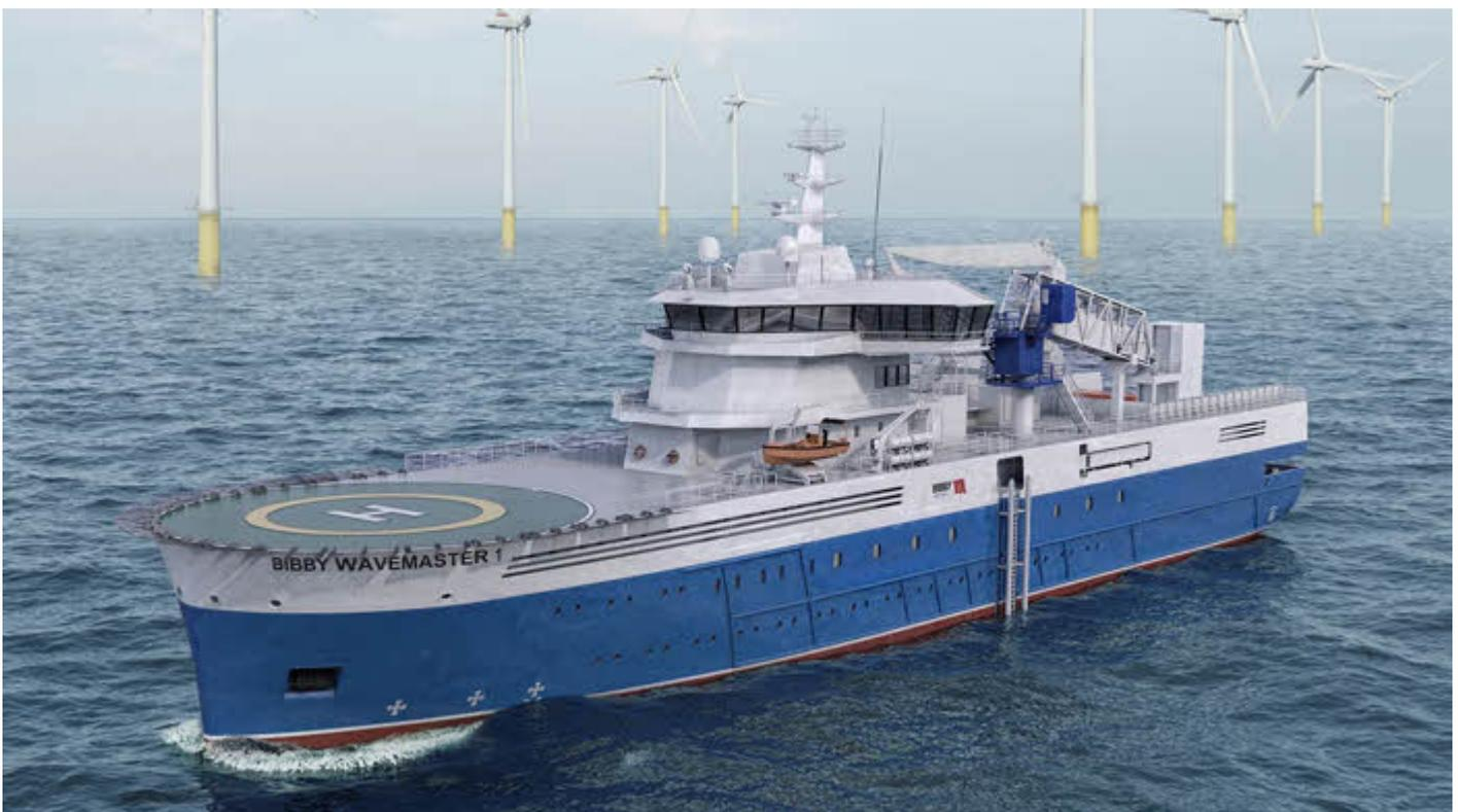
When delivered from the Damen Galati shipyard in Romania, it will be Bibby Marine's first vessel purpose-built for the transfer and accommodation of offshore personnel to wind farms being constructed deep offshore.
