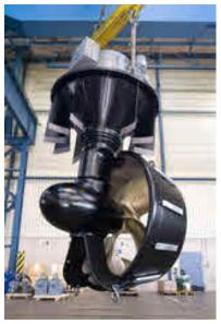
greater abrasion resistance and approx. 60% greater adhesion. For the above-water sections, Schottel uses a very dense and extremely durable two-component polyurethane coating.
